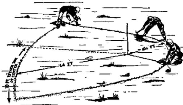
Figure 31. Fan type emplacement for 57-mm antitank gun.
