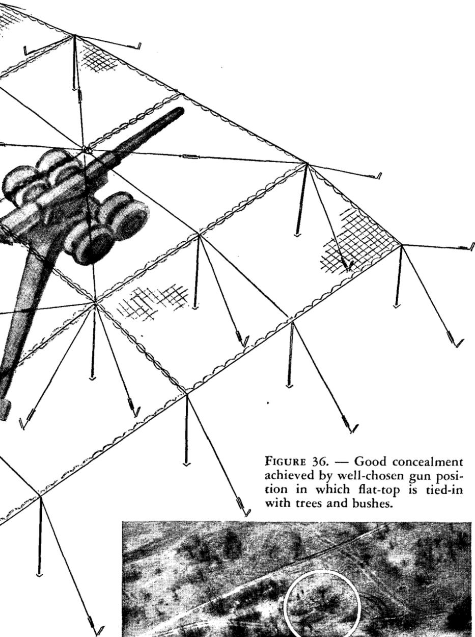
FIGURE 36. — Good concealment achieved by well-chosen gun position in which flat-top is tied-in with trees and bushes.
