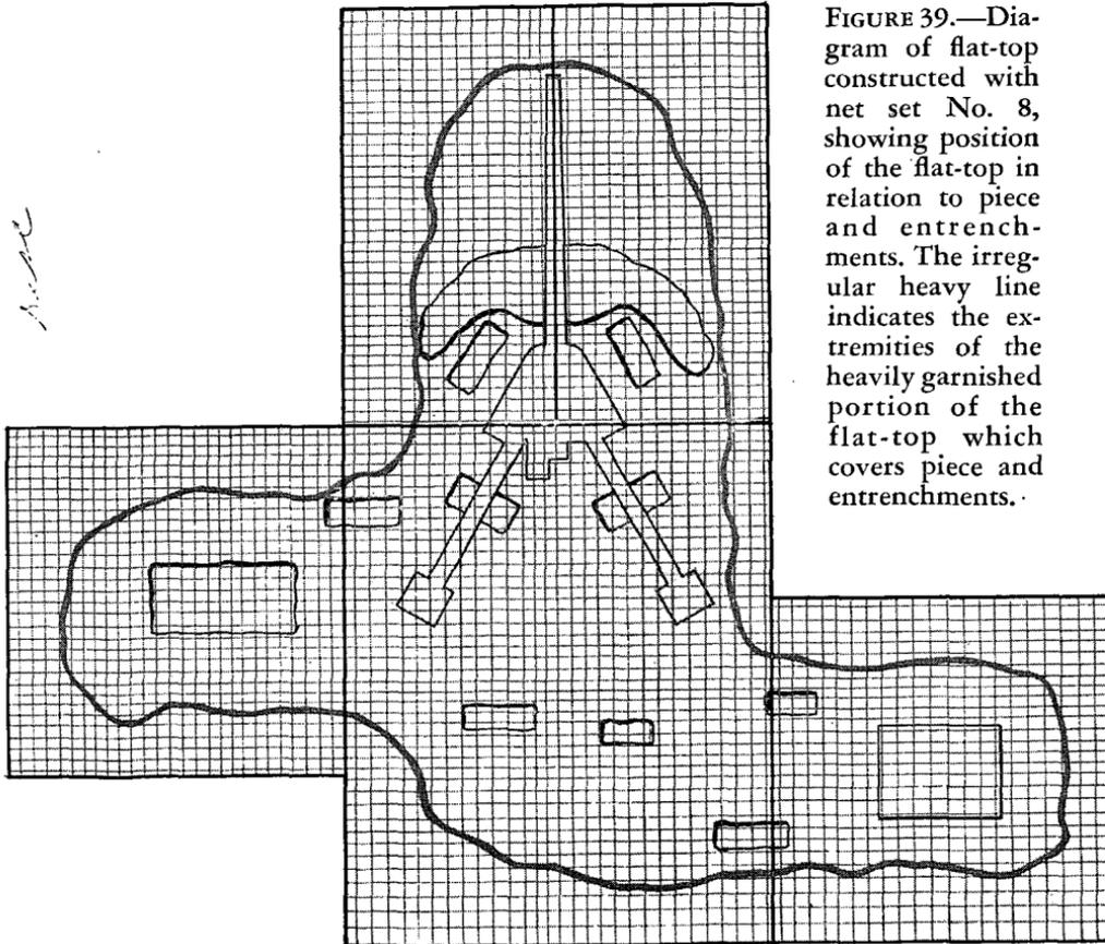
FIGURE 39.—Diagram of flat-top constructed with net set No. 8, showing position of the flat-top in relation to piece and entrenchments. The irregular heavy line indicates the extremities of the heavily garnished portion of the flat-top which covers piece and entrenchments.
