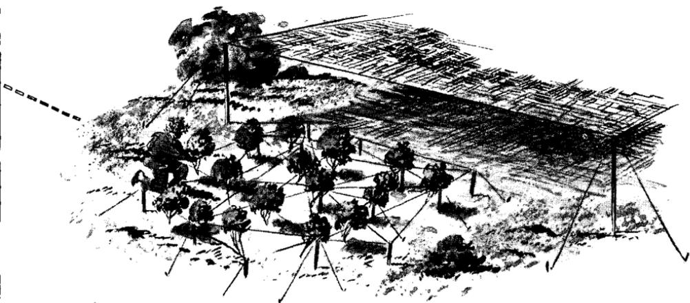
FIGURE 62 ④.—Blast marks can be concealed. One method of camouflaging blast marks is to cover area with network of wire supported on  $2\frac{1}{2}$ -ft. stakes. This network is used to support branches and other suitable foliage in natural position over blast mark area. The network should be irregular in outline and cover a larger area than the blast mark.
