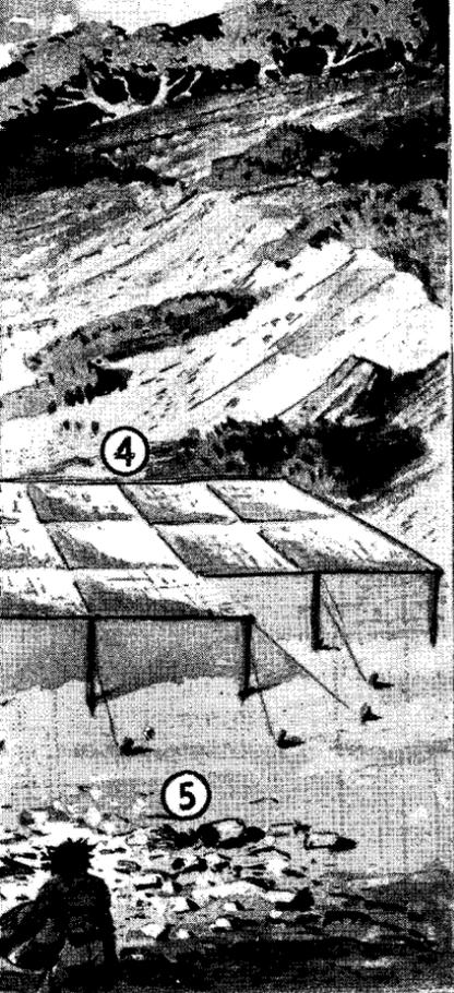
④.—Flat-tops must be kept flat and taut to prevent easily identified wire pattern from showing through. At night, when dew is expected, or during rain, twine nets must be slacked. When drying, nets must be tightened to keep flat and taut.
