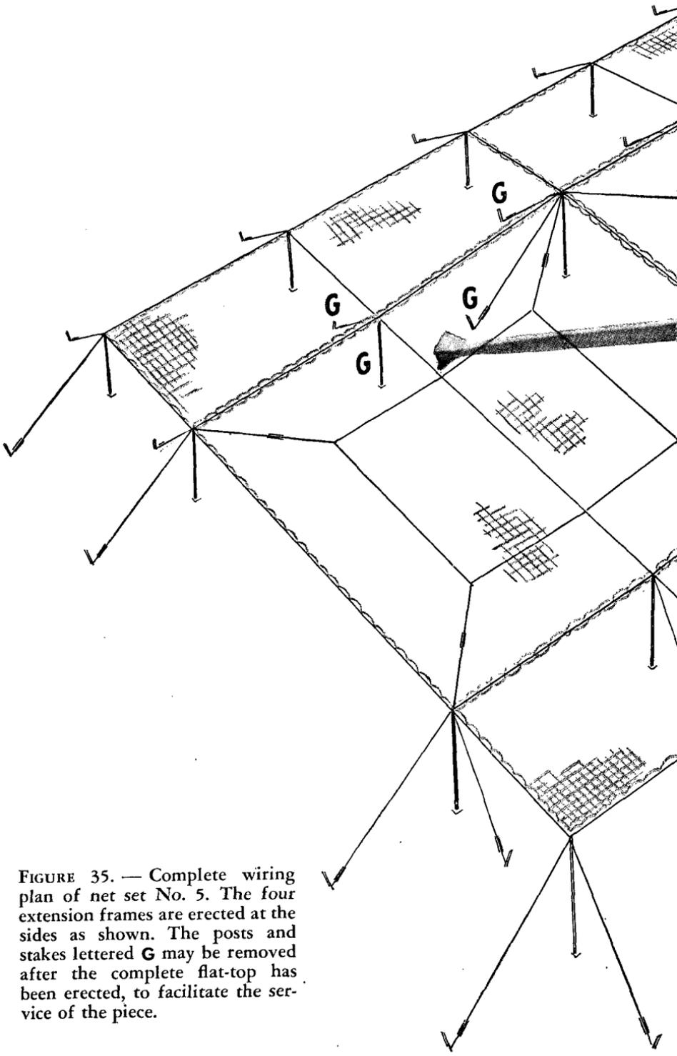
FIGURE 35. — Complete wiring plan of net set No. 5. The four extension frames are erected at the sides as shown. The posts and stakes lettered G may be removed after the complete flat-top has been erected, to facilitate the service of the piece.
