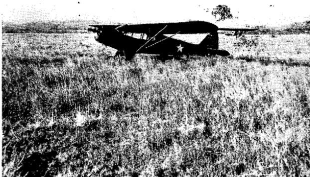
FIGURE 81. — Plane parked along a hedge line and covered with natural materials. The air view below shows that although plane is not completely concealed, it is almost lost in a natural line in the terrain and is likely to be overlooked. For complete concealment in this case, both the net and natural materials should be used.
