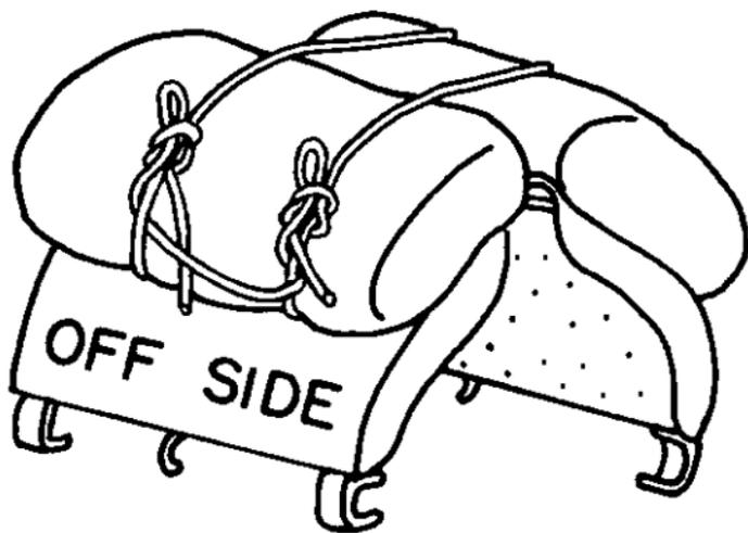
**FIGURE 29. Double-tie sling complete.**
