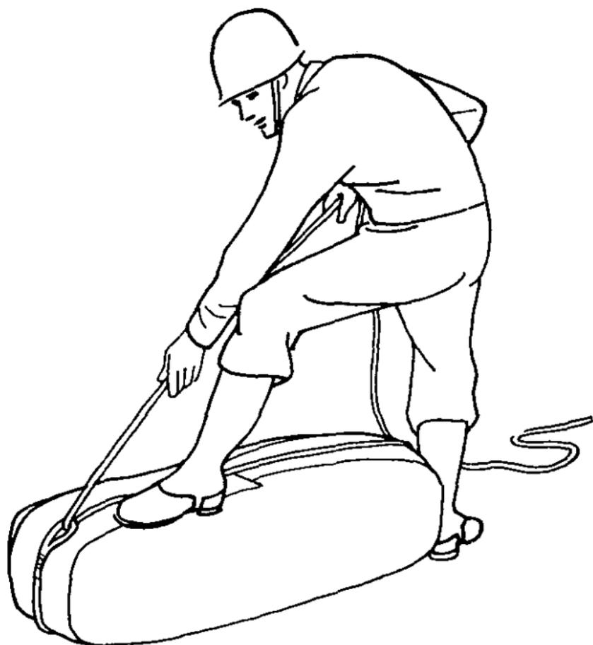
**FIGURE 13.** Tightening lengthwise loop.
