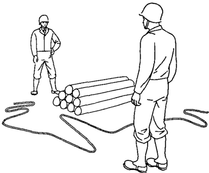
**FIGURE 19. "Z" rope formation for lairing cargo.**
