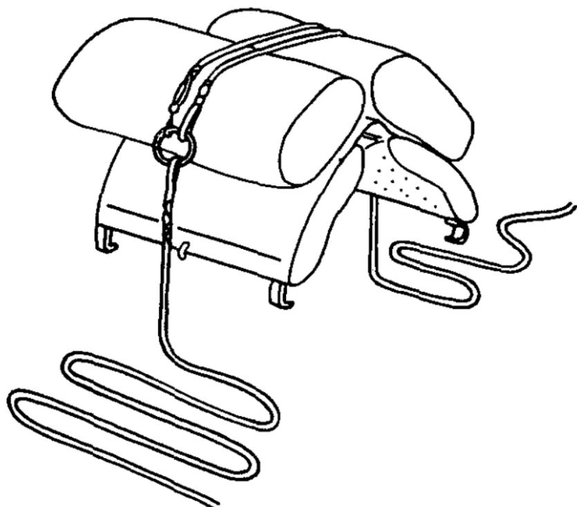
**FIGURE 69. Load cinch positioned (Sweeten diamond hitch).**
