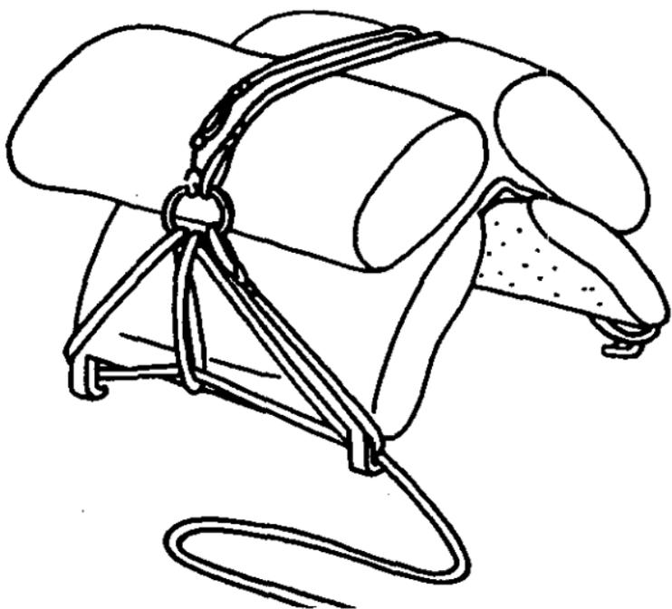
**FIGURE 71.** Second step in forming Sweeten diamond hitch.
