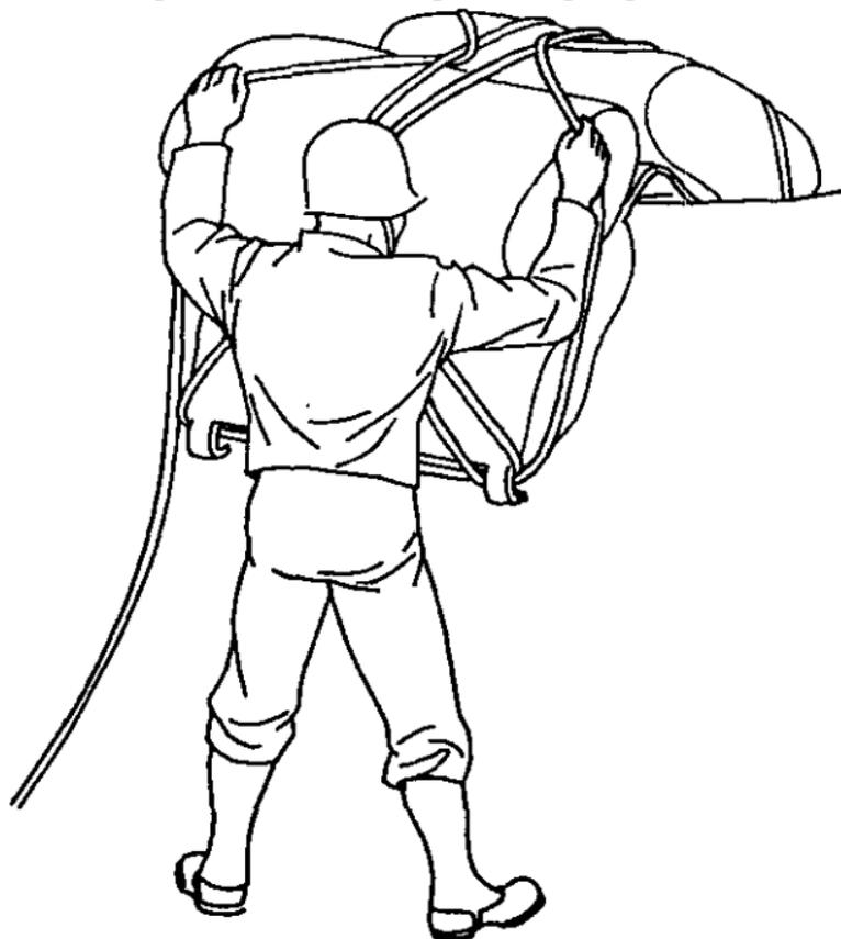
**FIGURE 74.** Holding tension on right quarter rope while taking slack on the running rope (Sweeten diamond hitch).
