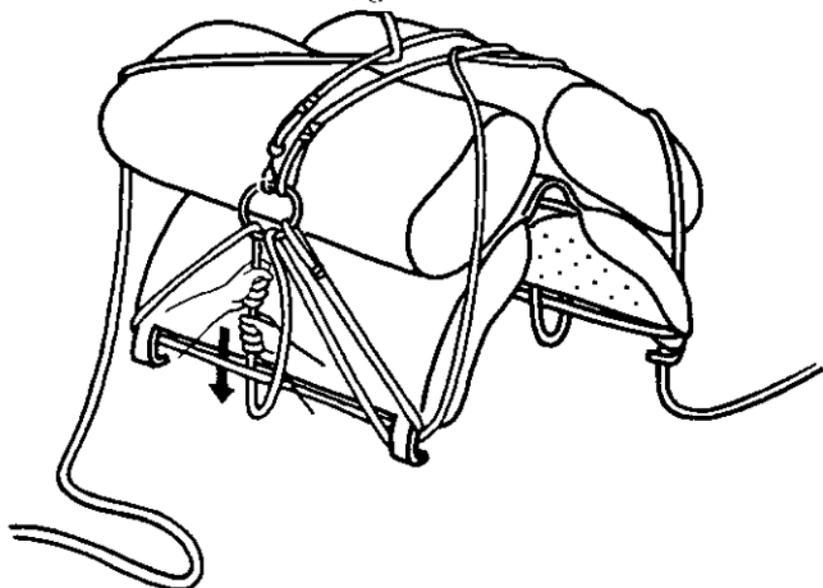
**FIGURE 73. First step in tightening Sweeten diamond hitch.**
