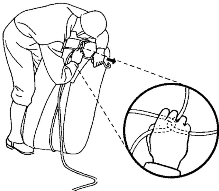
FIGURE 14. Adjusting first half hitch.
