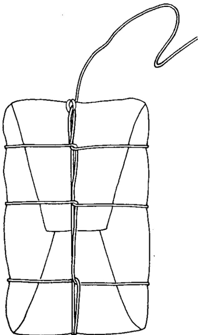
FIGURE 16. Half hitches in position.
