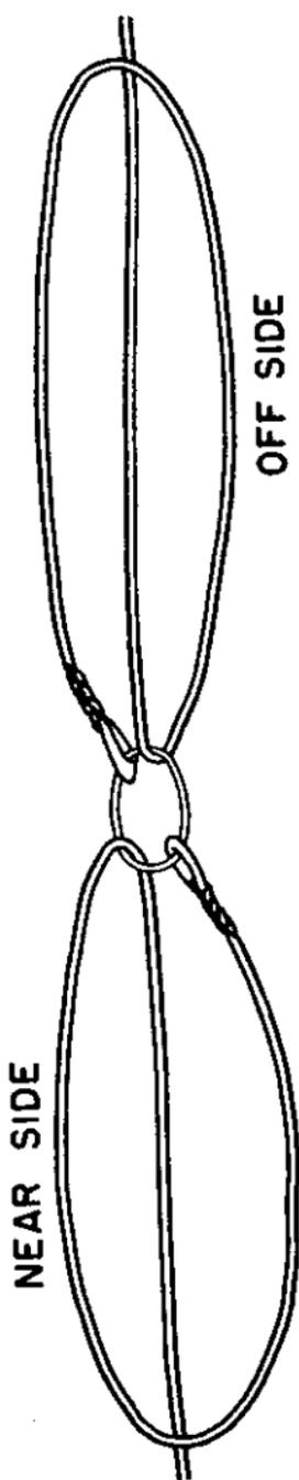
FIGURE 79. Loops formed for Nagle hitch.
