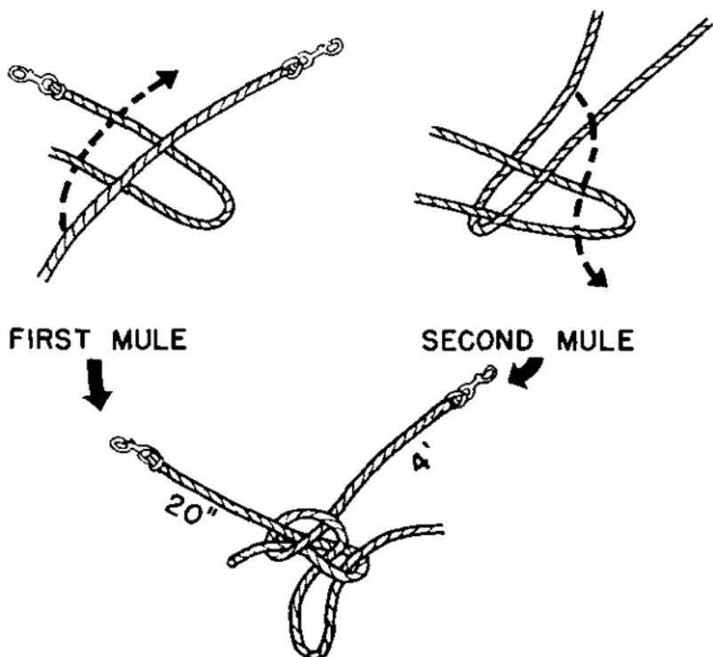
FIGURE 93. Floating picket line knot.
