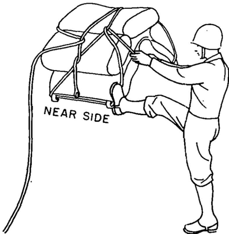
**FIGURE 60.** Near packer grasping running rope with both hands to remove all slack (double diamond hitch).
