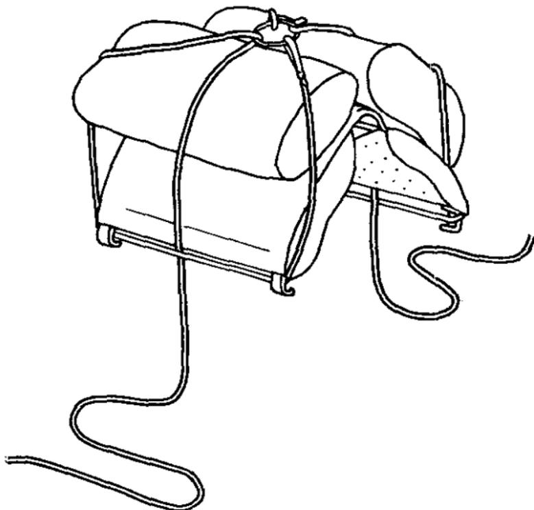
**FIGURE 80.** Loops in place on load (Nagle hitch).
