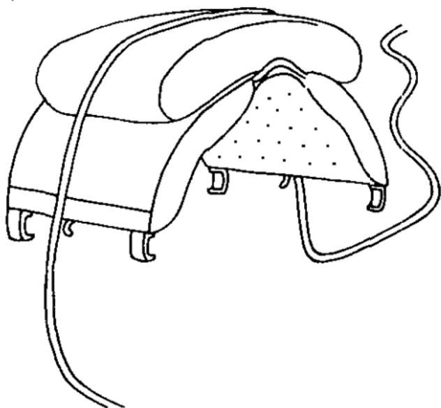
**FIGURE 35.** The first step in formation of squaw hitch.
