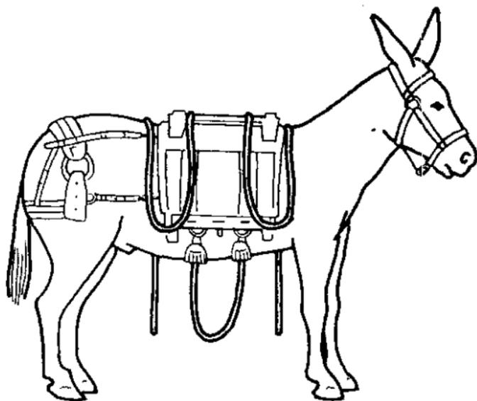
FIGURE 26. Adjustment of sling rope for cross-tie sling (alternate method).
