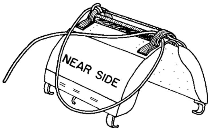
FIGURE 62. The initial formation of lash rope for basket hitch.
