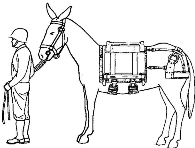
**FIGURE 9. Phillips pack saddle, cargo, in proper position.**
