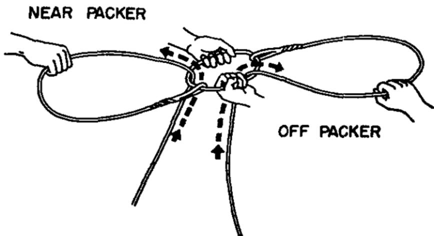
**FIGURE 78.** Forming loops for Nagle hitch.
