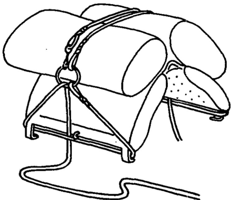
**FIGURE 70.** First step in forming Sweeten diamond hitch.
