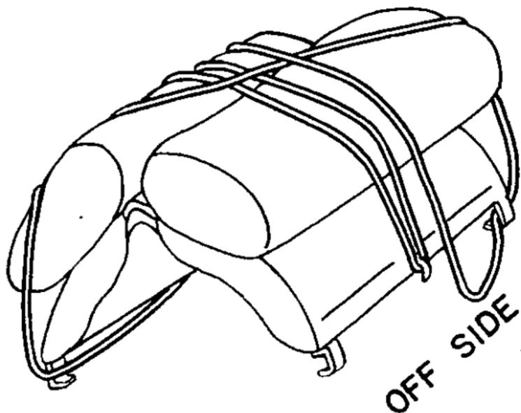
FIGURE 54. Formation of front quarter ropes (Phillips cargo hitch).
