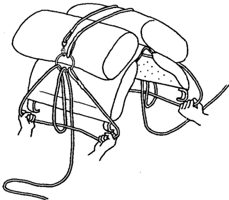
**FIGURE 77.** Second step in rapid formation of Sweeten diamond hitch.
