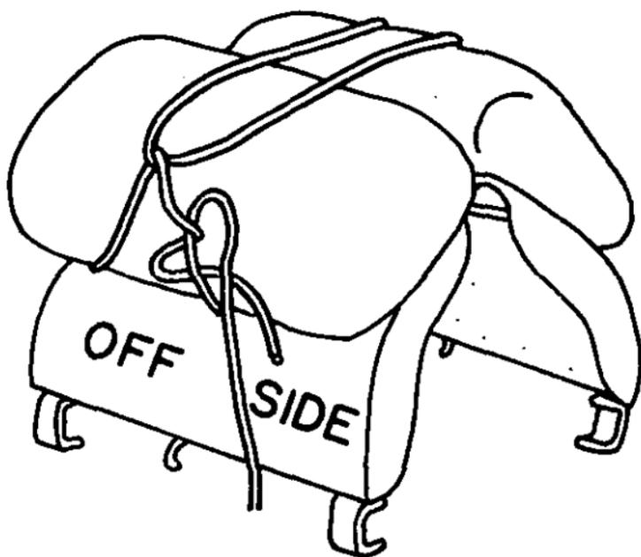
**FIGURE 31.** Single-tye sling complete except for square bowknot.
