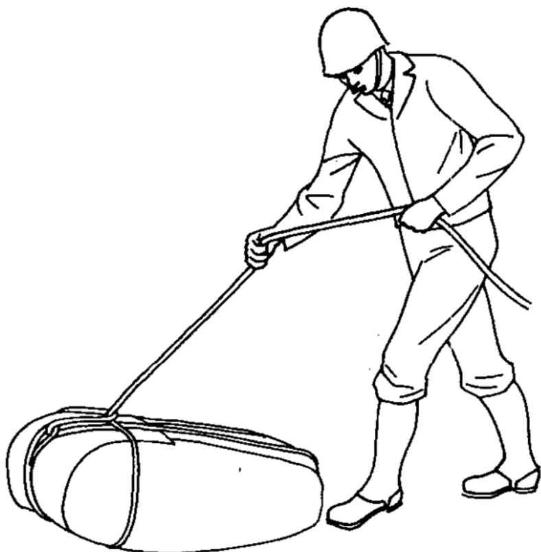
**FIGURE 15.** Tightening first half hitch.
