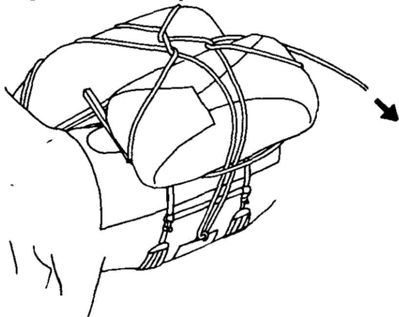
**FIGURE 111.** Wyoming diamond hitch formed and ready to be tied.
