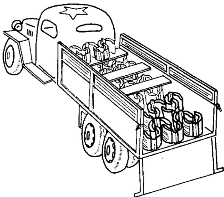
**FIGURE 6.** Pack saddles properly loaded in vehicle.
