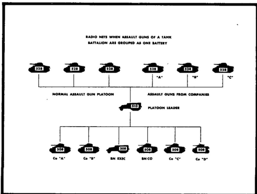
*Figure 4. The assault gun attached to the assault gun platoon enters the assault gun platoon net by selecting the proper channel on the SCR-528.*
