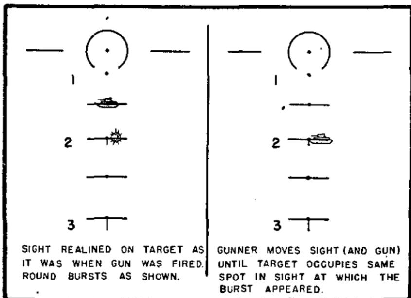
FIGURE 24.—Automatic correction method.
