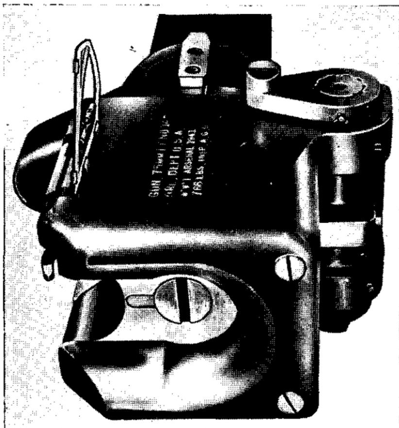
FIGURE 36.—Position of gunner's quadrant on breech ring. 75-mm tank gun M3.
