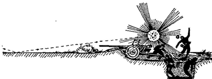
FIGURE 9.—Firing 75-mm shell, HE. With the fuze set at DELAY, a short bursts on ricochet. Ricochet bursts are deadly against personnel.
