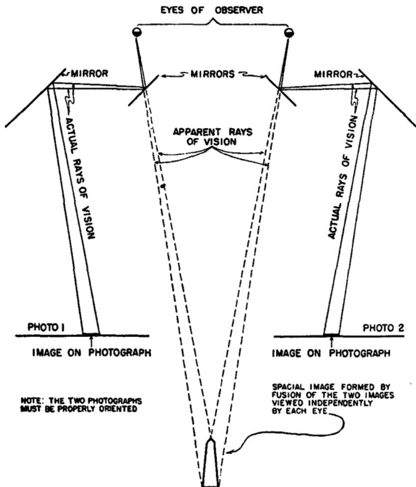
FIGURE 8.—Diagram showing stereoscopic perception.
