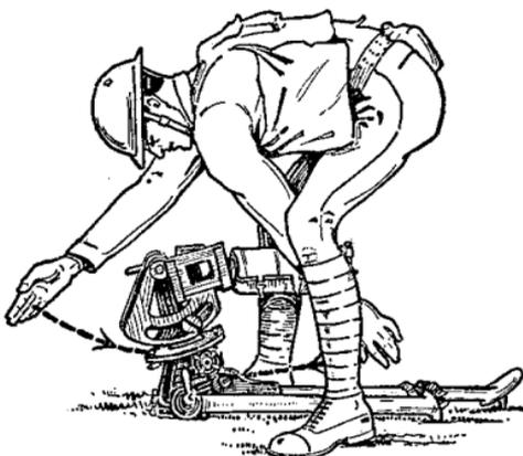
FIGURE 36.—Mounting the tripod
