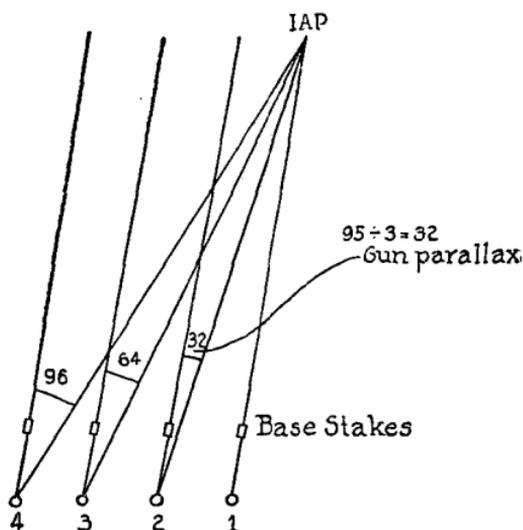
FIGURE 44.—Laying guns on parallel lines
