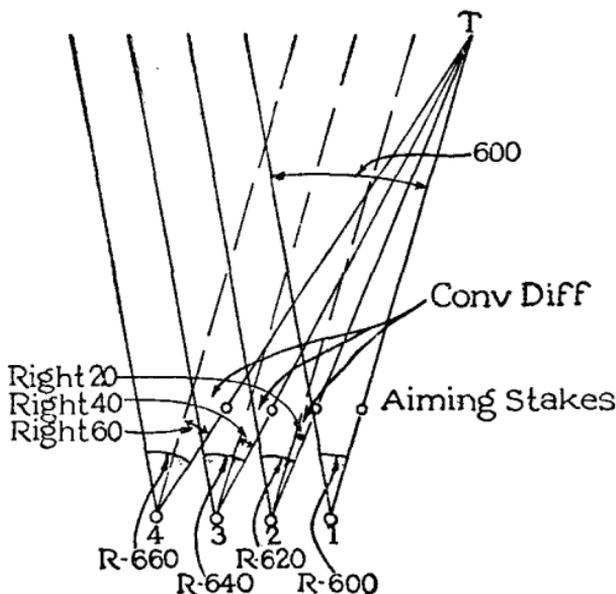
FIGURE 47.—Laying guns on a narrow or point target
