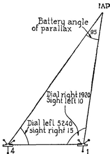
FIGURE 43.—Measuring the battery angle of parallax
