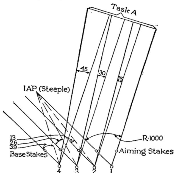
FIGURE 48.—Establishing base and direction lines
