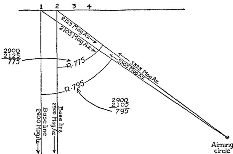
FIGURE 42.—Using the aiming circle or a compass as the initial aiming point
