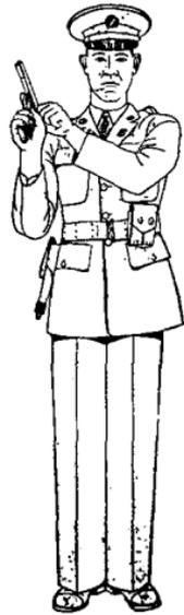
③ To pull the slide downward in loading.
