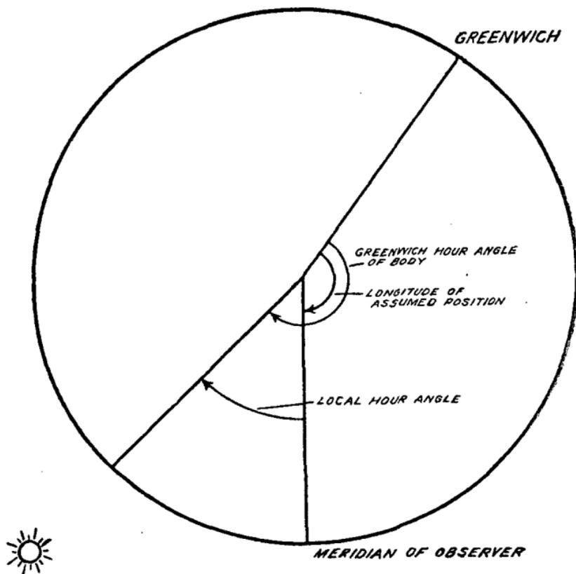
FIGURE 10.—Hour angle diagram.
