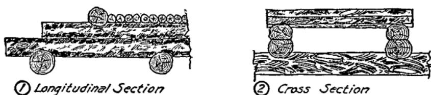
FIGURE 3.—Log culvert
